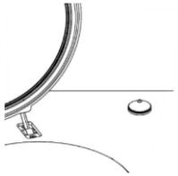
Figure 13 shows the steam vent opened. This operation is achieved by rotating the steam vent cover disc either clockwise or anti-clockwise on the top of the cooker.
