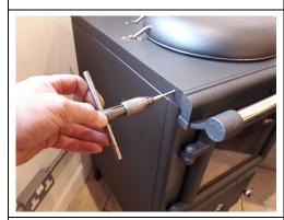
4. Use a M6 tap to add a thread to the drilled holes.
