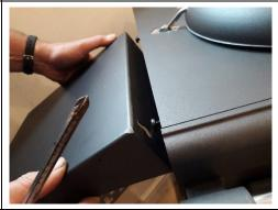
6. Offer the shelf up to the cookstove, dropping the keyhole slots in place, over the fixing bolts.
