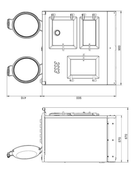
The cooker is not to be grouted or sealed at the back or sides of the worktop as if any maintenance is required the cooker will have to be pulled away from the wall at the rear. This is to allow the cooker top to be lifted.
