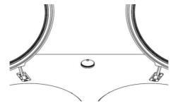
Figure 7 shows the steam vent opened. This operation is achieved by rotating the steam vent cover disc either clockwise or anti-clockwise on the top of the cooker.
