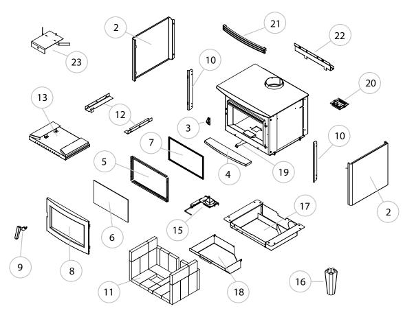
Figure 10. AB25.Exploded Parts.
