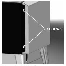
Figure 3. AB25. Side panel screws.
