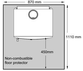
Figure 6. AB25 AUS Floor protection.
