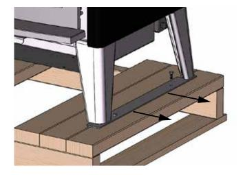
Figure 2. AB25 Hold down removal1.
