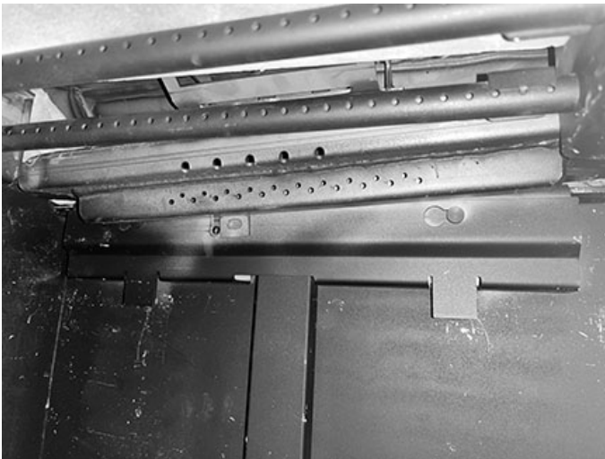
Figure 28. Remove rear baffle
