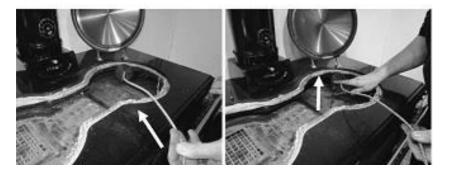
There are two methods to clean the right side flueway. The first is to insert the brush at a shallow angle as shown above. The brush will need to turn 90° into the flueway so steady pressure will be needed to help the brush head round the bend. Once in, work the brush up and down and front to back as the flue way runs along the entire depth of the ovens. Again, soot will fall into the trap between the ovens.
