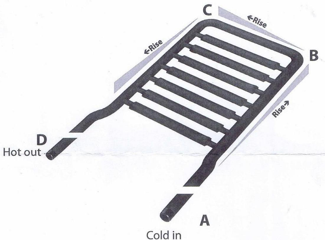
For correct venting, the Hotflow Unit **must** rise as shown above, once mounted.
