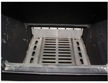
1) ALLOW THE FIRE TO GO OUT AND COOKER TO COOL DOWN, THEN CLEAR OUT THE FIRE BED
