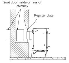
Fig. 6 Horizontal Register Plate With Rear Flue Connection
