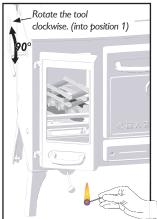
Open the flue gas diverter by pulling the tool forward. Build a stack of 6-8 softwood kindling sticks. This can be in grid shape or a pyramid with paper or firelighter in the centre, ensure to leave a space between the pieces to allow the air to circulate around and through them and light.
