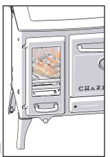
Add larger logs once fire is established. The air control can be reduced to the nominal click position. If cracked open, the door can now be closed. Set the flue diverter into the normal position 2 (push back).
