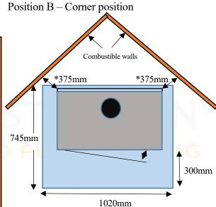
\*The side wall clearance can be reduced to 75mm from a combustible wall when the is appliance is fitted with side heat shields 50mm from each side of the appliance measuring 445mm wide x 1310mm high x 1.5 thick. The 75mm clearance from a combustible wall is measured from the rear corner of the appliance side heat shields.
